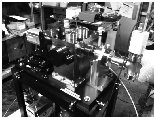
Figure 1. A grazing-incidence spectrometer for the plasmoid collision EUV light source.
