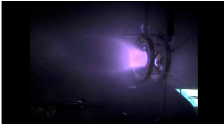
Steadily generated magnetized plasmoid by rotating magnetic field.
