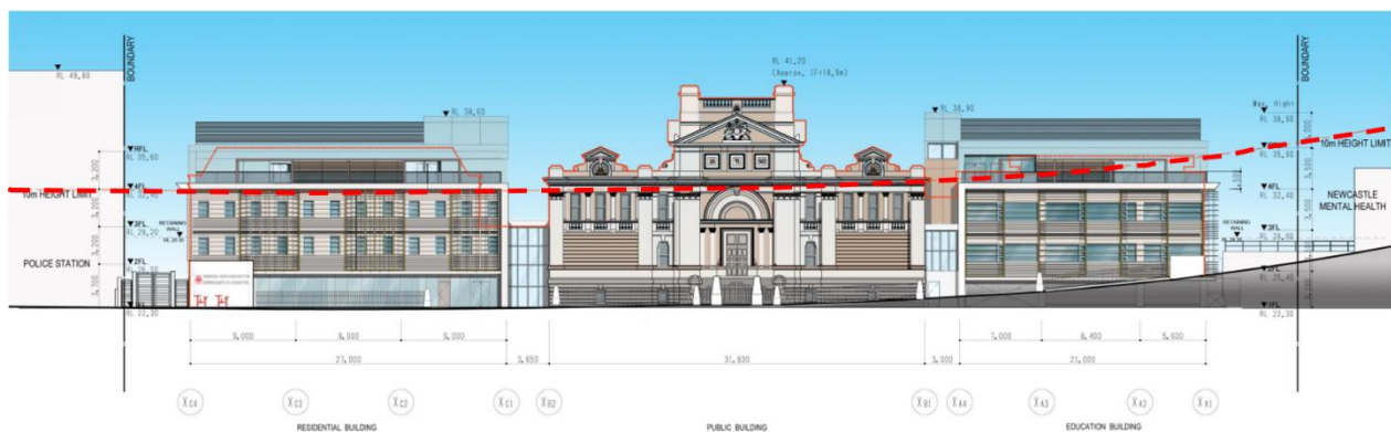
Figure 2: Northern elevation of proposed development showing outline of existing development with orange line and 10m height limit in red dotted line (Source: Azusa Sekkei)
