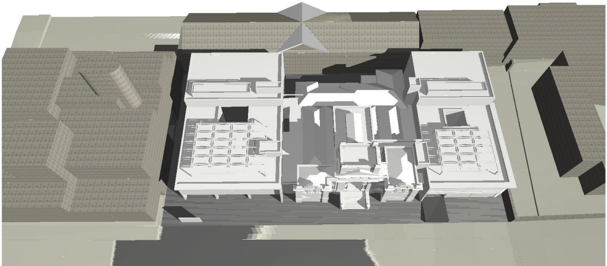
Figure 11: 3D Model showing shadow impact of proposed development at 3:00pm, winter solstice (Source: Azusa Sekkei)
