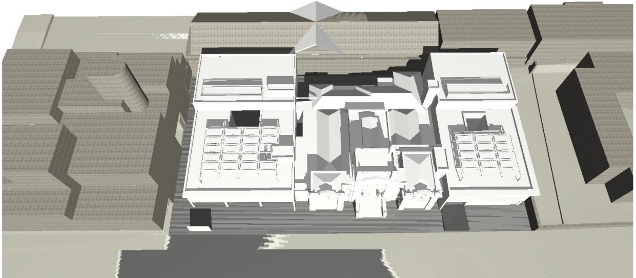
Figure 8: 3D Model showing shadow impact of proposed development at 12:00pm, winter solstice (Source: Azusa Sekkei)
